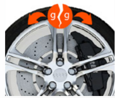
Split and hidden weight solution 平衡块分割隐藏功能
